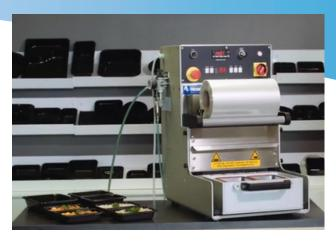
The moulds are quickly and easily changed without tools, making this machine suitable for many types of trays and film. The computer controlled sensor for vacuum and gas injection ensures the best possible shelf life at the quickest packing time.
